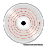
A digital disc stores information that is encoded in a long chain of 1s and 0s.
